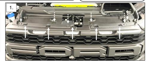
2. Fold up the rubber radiator shroud and disconnect all the electrical for the front grille. There will be a total of 4 connectors ( ⋪) and 3 plastic rivet push clips ( ⋪) .
